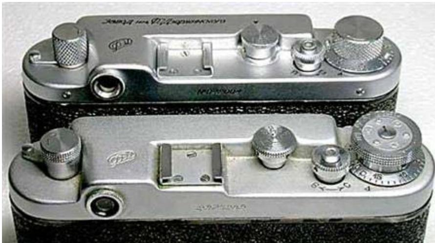
This photo contrasts a rear view of an early and a late model FED 2. Some of the differences include the later style 'mushroom' winder knob, with less knurling on both it and the rewind knob. The higher position of the accessory shoe on
